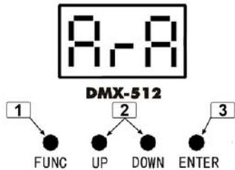
In the MODE OPTION setting, the stand alone laser show that you are going to choose is flashing. Press FUNC to change stand alone laser show, you will have 3 different stand alone preprogrammed laser show. Their DISPLAY and EFFECT are listed below:
